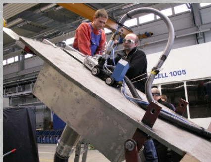
During cutting tests in 45° down position
