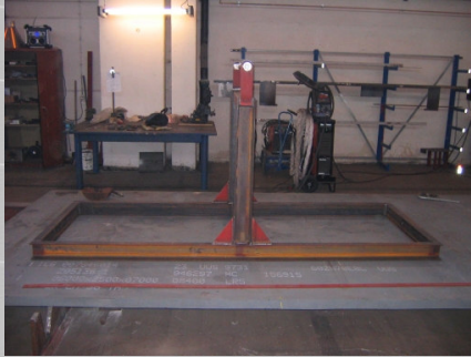
Device for turning the plate to simulate different cutting positions
