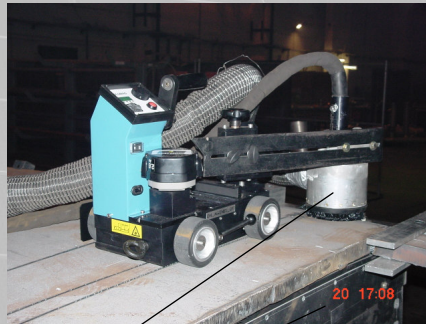
Plasma cutting with exhaust system above and below the plate
