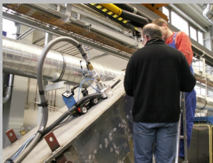
During cutting tests in 45° down position
