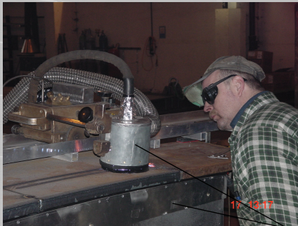
Plasma cutting with exhaust system above and below the plate
