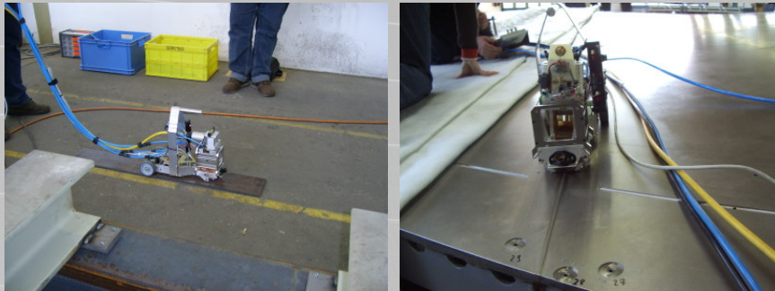
Tractor with laser welding head
