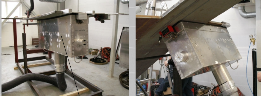
Beam catcher below the plate with exhaust system in different positions
